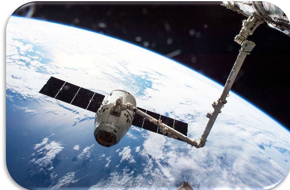
"Canadarm2 catching SpaceX's Dragon resupply ship as it arrives at the ISS in 2016"
